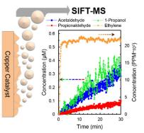
comparison to conventional gas chromaograph techniques, SIFT-MS can be used to fully analyze the voltage dependent performance of catalysts in hours as compared to days. The high time resolution of SIFT-MS will enable new insight into the mechanistic pathway of EC-CO2R that were previously inaccessible due to the lack of suitable analytical equipment.
