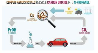
nanoparticles and were catalytically stable for at least six hours, with only a 14 per cent deactivation after 12 hours of reduction. With a very high octane number and energy density, n-propanol commands a higher market value than other CO<sub>2</sub> reduction products like methane. It can also be blended with gasoline to deliver clearer burning fuel with lower greenhouse gas emission, making the discovery a boon for the energy industry.
